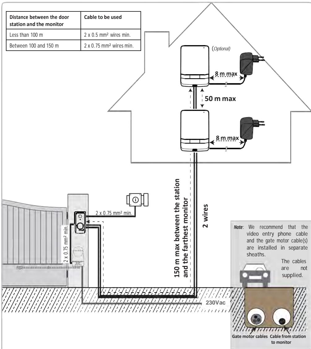
**Note:** If you need to use junction boxes to cable the video entry phone, do not use more than two boxes between the station and the monitor, or more than one box between the monitor and the power plug.
