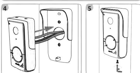
[5]. Screw the door station to the rain shield using the tamper-proof torx key provided.
