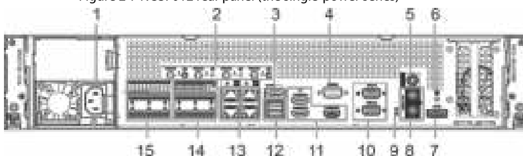
Figure 2-8 IVSS7012 rear panel (the redundant series)
